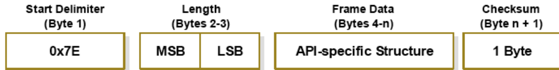
Figure 4-01. UART Data Frame Structure:
