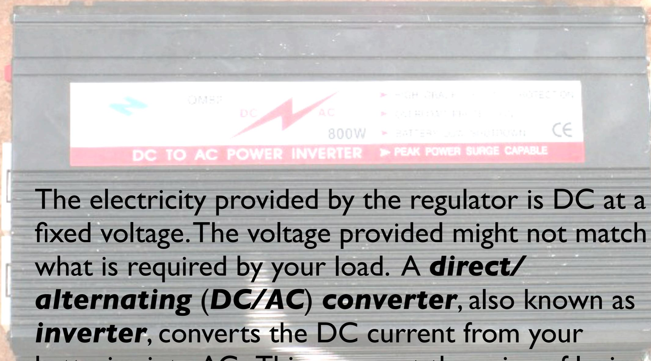
The electricity provided by the regulator is DC at a fixed voltage. The voltage provided might not match what is required by your load. A **direct/alternating (DC/AC) converter**, also known as **inverter**, converts the DC current from your batteries into AC. This comes at the price of losing some energy during the conversion.
