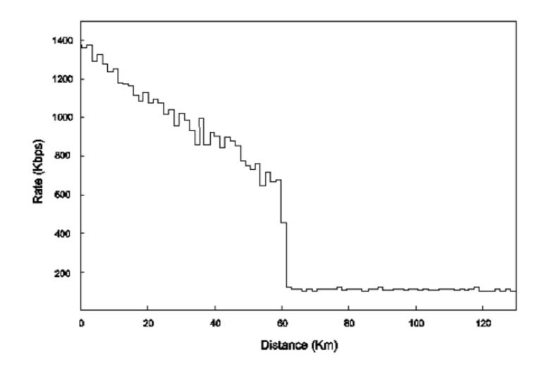
Rate versus distance for an FTP file transfer, simulated with NS2
