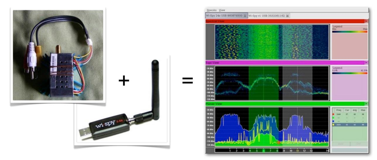
The ideal antenna alignment toolkit consists of a **signal generator** and a **spectrum analyzer**, preferably one of each at both ends of the link.
