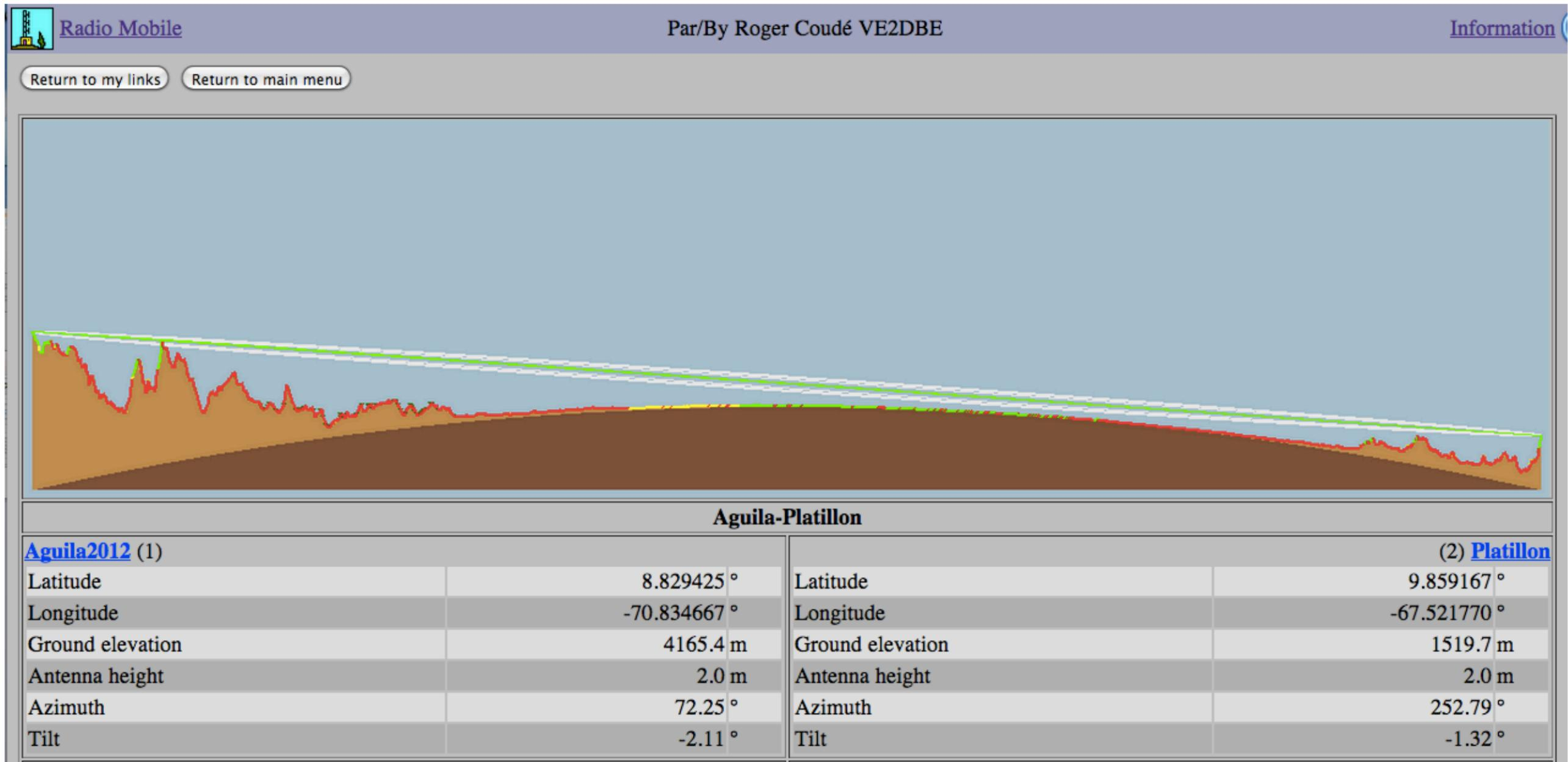
This link has a clear line-of-sight and a free Fresnel zone, shown as the white curved line surrounding the straight green line. Notice that the antenna tilt is negative at both ends, despite the fact that one end is much higher. This is because the radio beam is curved due to the refraction introduced by the atmosphere.
