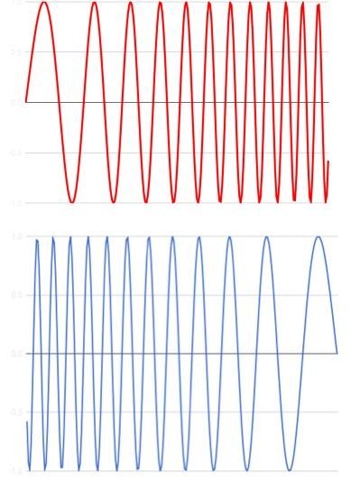
Up-chirp: sinusoidal signal of linearly increasing frequency
