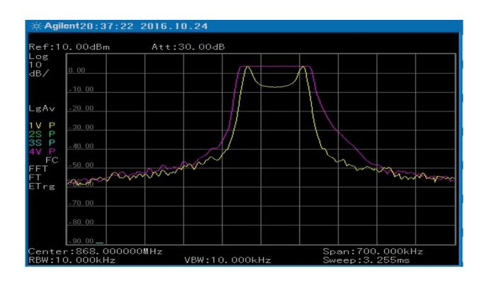
Flat top LoRa spectrum implies a more efficient spectrum usage as compared with the two peaked FSK.
