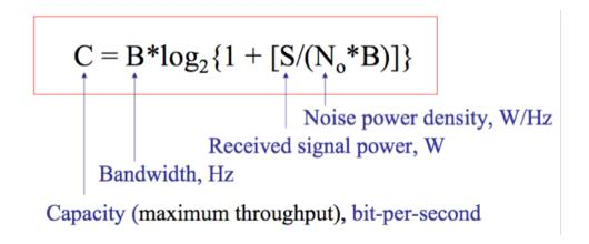
The maximum range is determined by the energy per bit received, and depends on the effective transmitted power, receiver sensitivity, interference and data rate.
