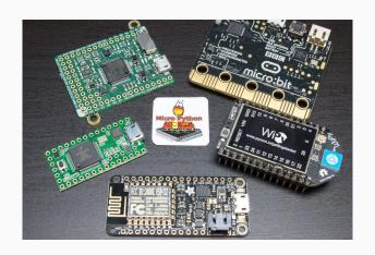
The MicroPython **pyboard** is a compact electronic circuit board that runs MicroPython on the bare metal, giving you a low-level Python operating system that can be used to control all kinds of electronic projects.
