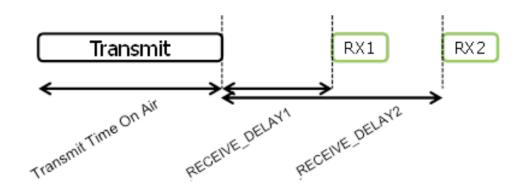
RxDelay1 is configurable, default is 1s. RxDelay2 default is 2s. First receive window data rate is the same as that of the last uplink by default, but it is region specific.
