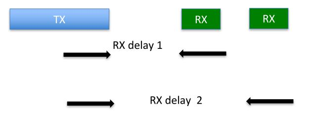
Class A : Following upstream transmission two receive windows are opened after the delay to account for the transmission times.
