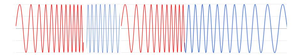
Data is conveyed in the transitions from upchirp to down-chirp and vice versa Tolerant to frequency drifts
