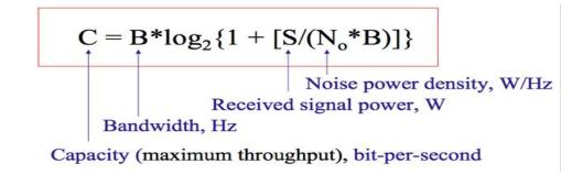
Capacity depends on the width of the channel in Hz, the received power and noise
