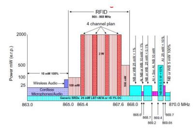
G1: 868,000 MHz to 868,600 MHz with 25 mW EIRP (14 dBm) and 1 % duty cycle. G2: 868,700 MHz to 869,200 MHz with 25 mW EIRP (14 dBm) and 0,1 % duty cycle. G3: 869,400 MHz to 869,650 MHz with 500 mW EIRP (27 dBm) and 10 % duty cycle.
