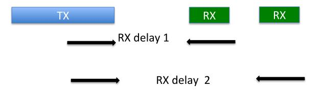
Class A optimized for battery power For low latency, use class B For no latency, class C
