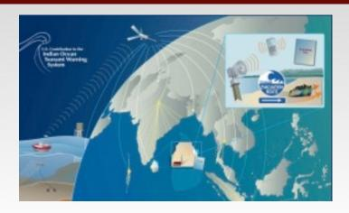
Early warning systems use kinetic sensors (measuring waves and water flow) are placed on the ocean floor and communicate data on potential tsunamis to disk buoys floating on the ocean surface via acoustic telemetry
