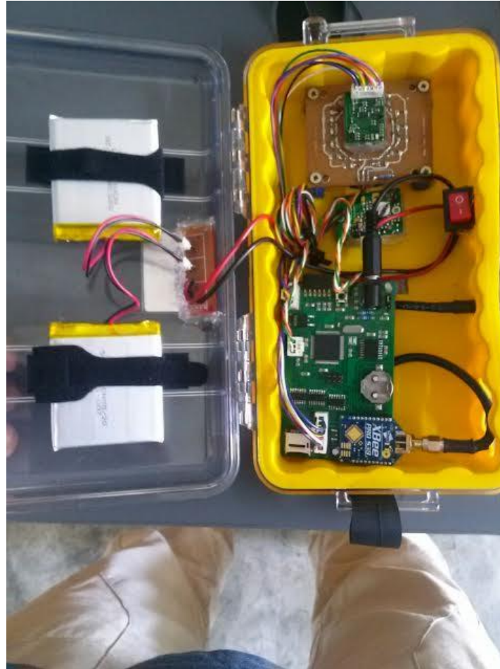
TapirDuino inside view.
