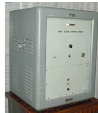
Figure 1.17: 1954 "DATRAC" 11-bit, 50-kSPS Vacuum Tube ADC Designed by Bernard M. Gordon at EPSCO
