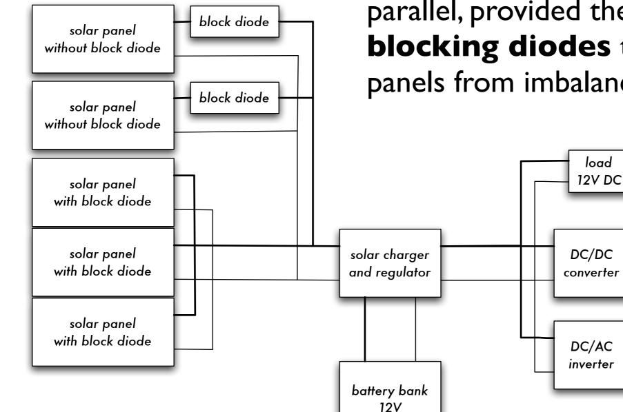
If more power is required, multiple solar panels may be joined in parallel, provided there are blocking diodes to protect the panels from imbalances.
