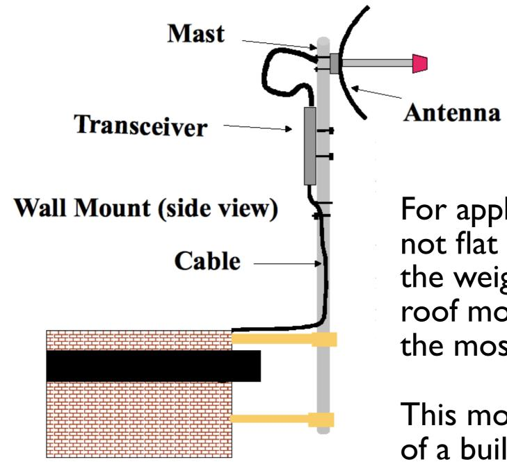
For applications where the roof is not flat or strong enough to hold the weight of a non-penetrating roof mount, the **wall mount** is the most effective solution.
