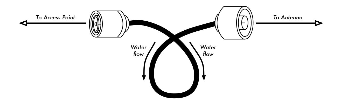
By adding a small loop to antenna and Ethernet cables, you can direct rainwater to flow away from the connector. This can greatly extend the life of your equipment.
