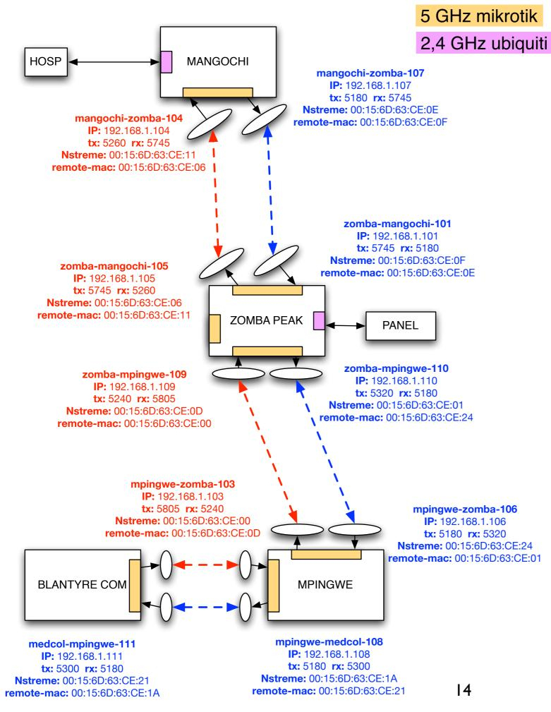
Here is an example of a network plan, with IP and MAC addresses, host names, locations, interconnections, operating bands, and frequency choices.
