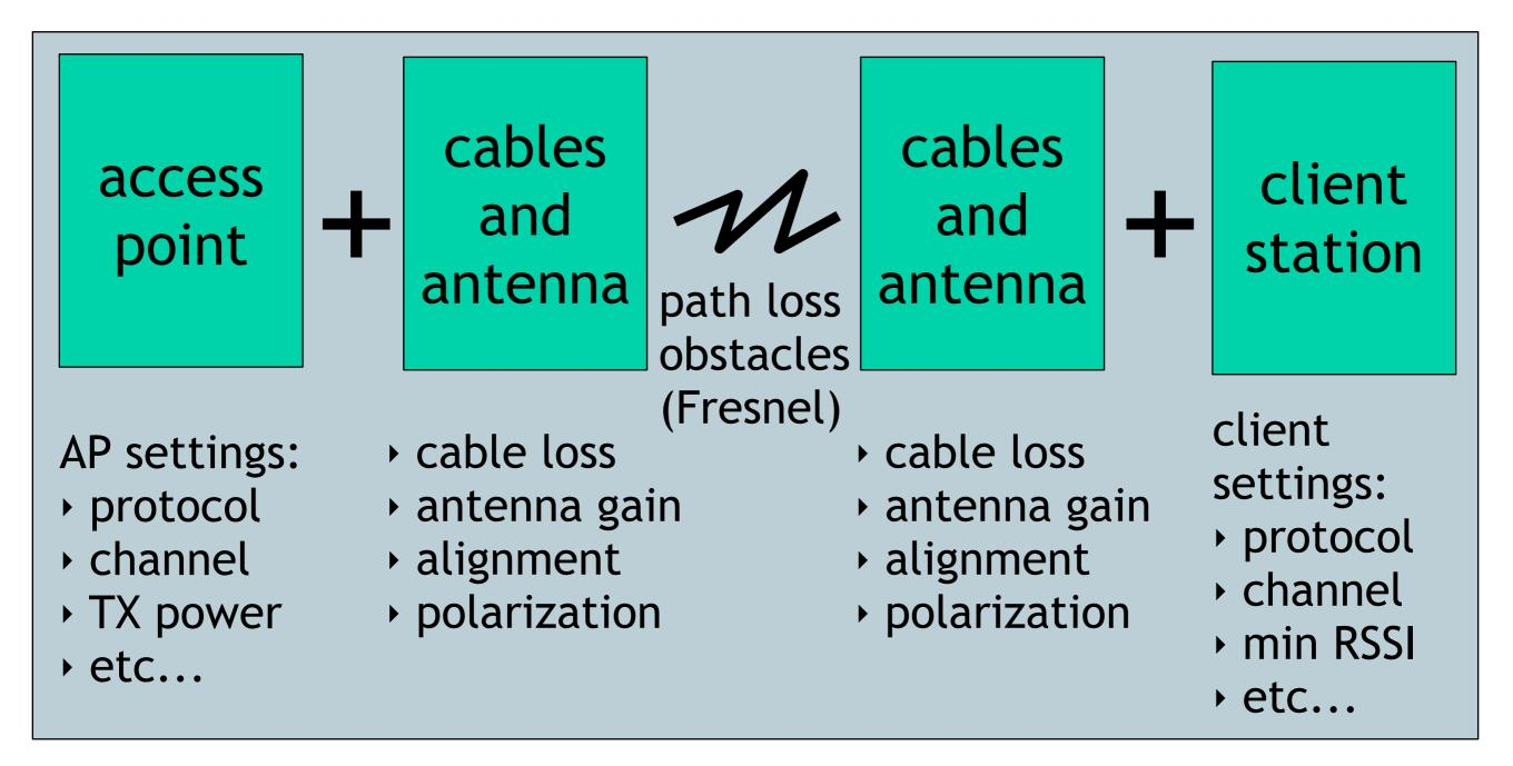
In order to have a working link: all relevant settings should match AND the link budget should allow for it
