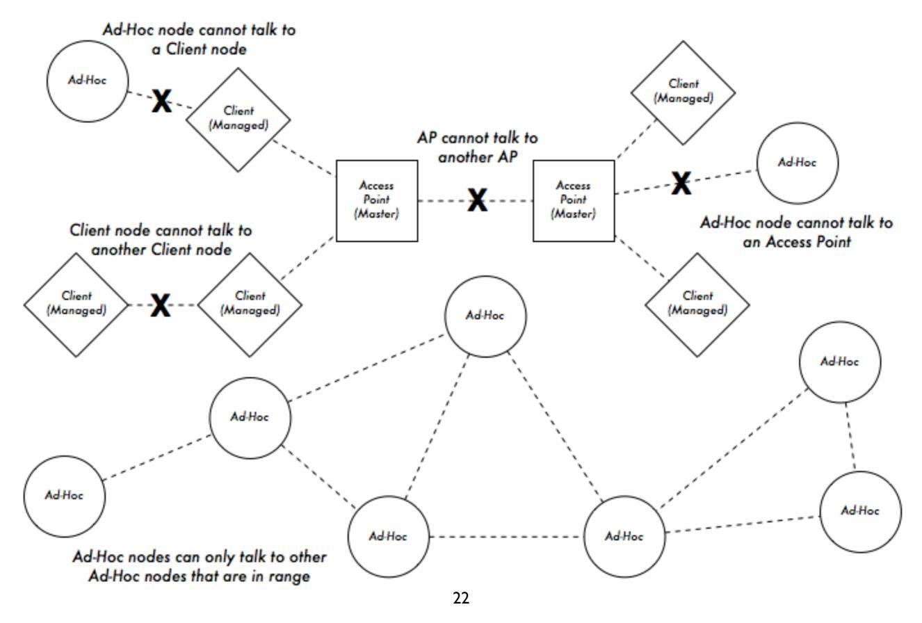
Access points cannot communicate with other access points over the air.A feature of WiFi called WDS (Wireless Distribution System) can allow up to five APs to communicate with each other via wireless, but throughput is greatly reduced, and vendor interoperability problems are common, so relying on it is generally discouraged.
