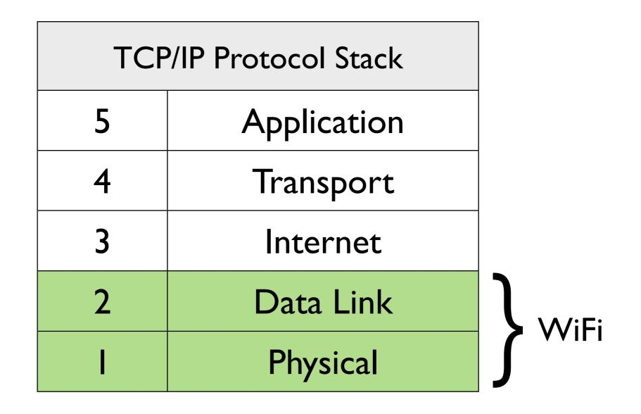
Complex networks use some kind of routing protocol to relay traffic between nodes.WiFi only provides a link-local network connection, up through TCP/IP layer two.
