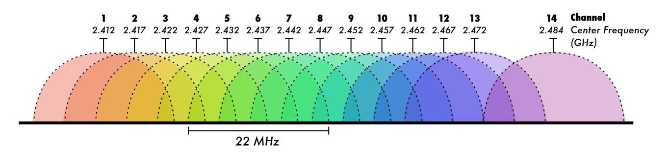
WiFi devices must use the same channel in order to communicate with each other. They send and receive on the same channel, so only one device may transmit at any time. This kind of connection is called **half-duplex**.
