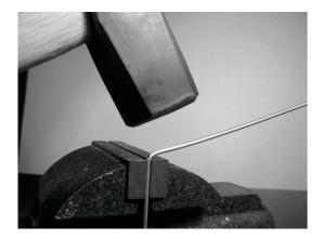
6) With a marker, draw a line at 3.05 cm from the edge, and bend the wire at 90 degrees in this point with the vice and the hammer as before, but in the opposite direction (it should look like a 'Z').
