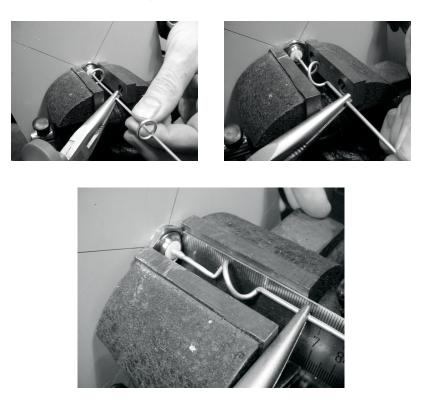
12) Repeat the same procedure for the other three coils, stretching their length to 2.0  $\rm cm$
