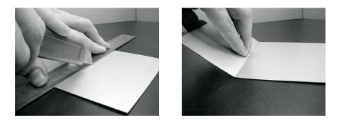
3) The edges can be now very sharp. Be careful when handling the plate. Use the file to smooth the edges all around.
