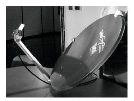
The construction is the same as the stand-alone Biquad antenna, but the shape of the metallic plate is different. The reflector has two side 'lips' which are 3 cm high, used to minimize coupling with the mounting bar of the feeder. These lips cut down radiation from the rear lobes of the biquad.
