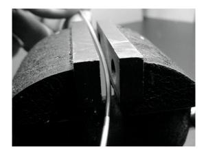
2) Cut the metallic plate to have a square shape of 12.3x12.3 cm. To do this, you may use the saw, but we suggest to use a thin (0.8 to 1.5 mm) aluminum plate, which can be cut with a cutter. Draw the correct dimensions on both sides of the plate with a marker. Carve the drawn lines with the cutter pressing firmly, helping yourself with the ruler. Do this a couple of times, on both sides of the plate. Bend the plate over the lines until it breaks.
