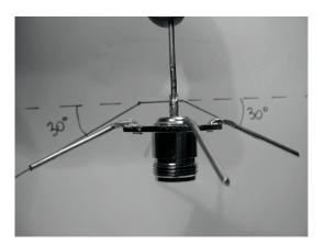
10) Trim the radial at a length of 3,05 cm measured from the corner of the flange. Smooth the end of the wires with the file.
