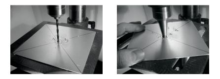
The hole should fit exactly the N connector. Use the file if needed.
