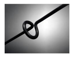
5) You should make a second coil at a distance of 7.8 cm from the first one. Both coils should have the same turning direction and should be placed on the same side of the wire. Make a third and a fourth coil following the same procedure, at the same distance of 7.8 cm one from each other. Trim the last phased element at a distance of 8.0 cm from the fourth coil.
