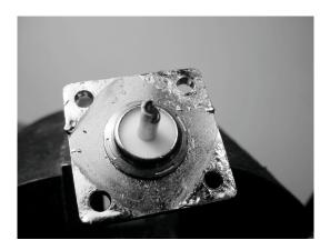
4) Smooth with the file one side of each of the wires. Tin the wires for around 1 cm at the smoothed end, using the high power soldering iron.
