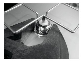
Rotate the nut so that the diagonals of the two wire squares are parallel to the side of the metallic plate. Then screw it firmly with the spanner.
