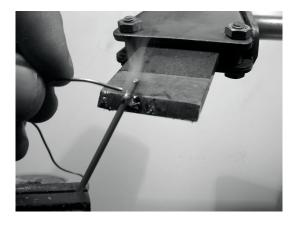
5) Bend at 90 degrees 0.5 cm of the tinned side of the wires with the pliers. Do it for four of the wires, leaving one straight. Help yourself with the vice and the hammer.
