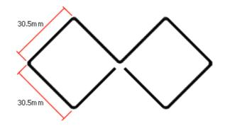
Bend the wire at 90 degrees in his central point using the vice and the hammer.
