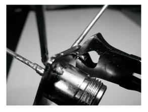
9) With the pliers, bent over the four radials at 30 degrees from the horizontal plane. This is done to match the impedance to 50 Ohms. To facilitate this operation, you may draw the 30 degrees angle on paper, and compare the antenna with it as shown.
