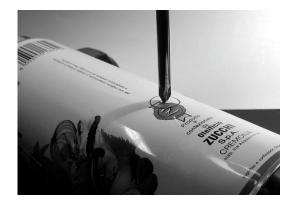
3) With a small diameter drill bit, make a hole at the center of the plate. Increase the diameter of the hole using bits with an increasing diameter. The hole should fit exactly the N connector. Use the file to smooth the border of the hole and to remove the painting around it in order to ensure a better electrical contact with the connector.
