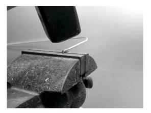
3) Draw another line at a distance of 3.6 cm from the bend. Using the vice and the hammer, bend once again the wire over this second line at 90 degrees, in the opposite direction to the first bend but in the same plane. The wire should look like a 'Z'.
