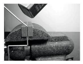
8) Draw now a line at 3.05 cm from the last edge, and a second line after 2.3 cm from the first one. Bend the wire at 90 degrees in the second line, in a direction orthogonal to the plane containing the wire, as shown.
