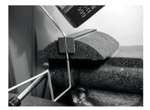
9) Bend the wire at 90 degrees in the first line drawn in the previous step in order to "close" the square, as shown.
