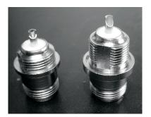
The central pin of the long type may be soldered directly on the shaped wire, while the short type of connector needs ad additional short piece of straight wire to be soldered into the central pin.
