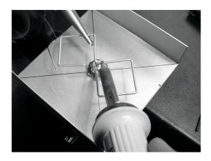
The procedure to fit the Biquad on the mounting bar may vary according to the shape of the original LNB fitting provided with the Parabolic Dish. It is usually round shaped, so it may be possible to use a rubber or plastic ring around the N connector to fix the Biquad in place.
