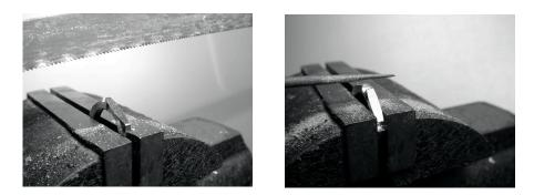
Be careful not to cut too deeply inside the nut: enough metal should remain to ensure its robustness.
