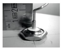
11) We are now going to stretch the coils extending the total vertical length of the wire. Using the use the vice and the pliers, you should pull the cable so that the final length of the coil is of 2.0 cm.
