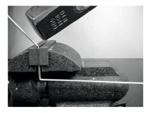
7) Draw another line at 3.05 cm from this new edge, and bend the wire at 90 degrees in this point, in the same direction as before.
