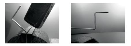
4) We will now twist the 'Z' portion of the wire to make a coil with a diameter of 1 cm. To do this, we will use the pipe or the drill bit and curve the wire around it, with the help of the vice and of the pliers.
