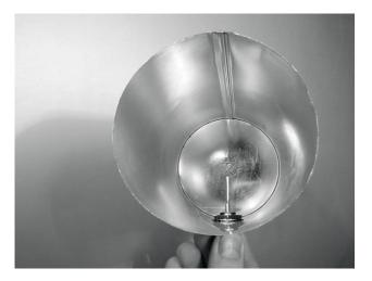
9) It is also possible to use an N-type chassis mount female connector with four-holes flange, that will make the building procedure someway more complex. In addition to the central hole, you should drill four more small holes to accommodate the screws necessary to fix the connector.
