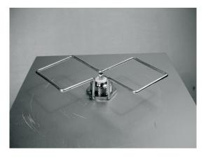
17) We now want to solder the central pin of the connector to the center of the shaped wire. You may have either a short or long type of N connector, as shown.
