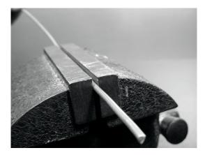
2) With a marker, draw a line at 2.5 cm starting from one end of the wire. On this line, bend the wire at 90 degrees with the help of the vice and of the hammer.
