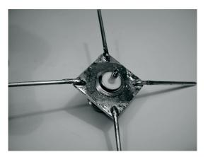
7) With the low power soldering iron, tin the central pin of the connector. Keeping the straight wire vertical with the pliers, solder its tinned side in the hole of the central pin.
