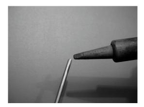
5) With the soldering iron, tin the central pin of the connector. Keeping the wire vertical with the pliers, solder its tinned side in the hole of the central pin.
