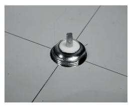
7) To have an antenna impedance of 50 Ohms, it is important that the visible surface of the internal insulator of the connector (the white area around the central pin) is at the same level as the surface of the plate. For this reason, cut 0.5 cm of copper pipe with an external diameter of 2 cm, and place it between the connector and the plate.
