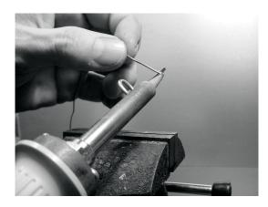
10) With the soldering iron, tin the central pin of the connector. Keeping the wire vertical with the pliers, solder its tinned side in the hole of the central pin. The first coil should be at 2.0 cm from the plate.
