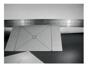
The lines between the central square and the two side rectangles should not be carved deeply on both sides with the cutter, but only on the upper side and just enough to facilitate the bending of the plate. The two lips should be folded at 90 degrees. Use the vice if needed.
