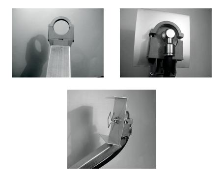
Other types of home-made directive antennas may be used as feeders for Parabolic Dishes. The important point is to match the beamwidth of the feeder with the dish size, and to place the feeder exactly in the focus of the dish.
