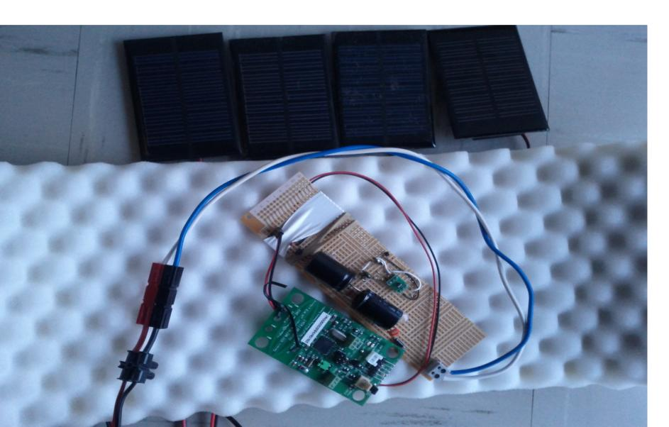
Wind and Barometric pressure at Barrvägen 2 Sensor Node 000d6 Powered via solar-charged 12V Lead-Acid battery
