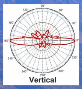
A self supporting tower very often has a tapered design, becoming narrower with height. This will uptilt the beam of a side attached omni up to 5 degrees. A typical 15 dBi omni has an 8 degree vertical beamwidth. The beam can be tilted upwards so much as to send all the signal where it does no good.
