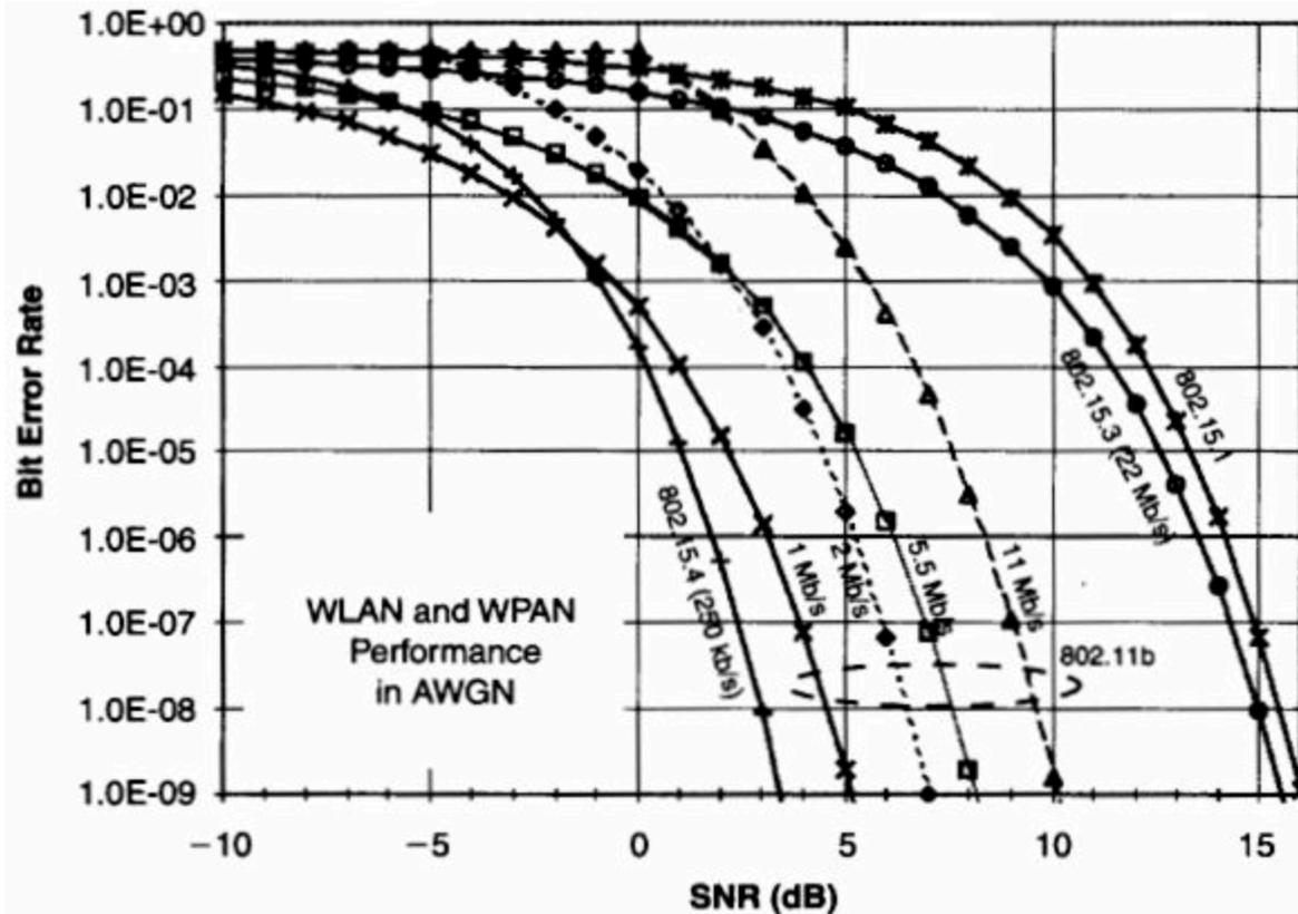
BER versus SNR for the four data rates of WiFi (IEEE 802.11b) along with values for Bluetooth (IEEE 802.15.1), WiMedia (IEEE 802-15.3) and ZigBee (IEEE 802.15.4), all operating in the 2.4 GHz band
