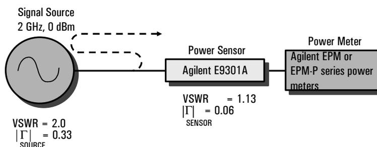
$$\text{Mismatch Uncertainty} = \pm 2 \times |\Gamma|_{\text{SOURCE}} \times |\Gamma|_{\text{SENSOR}} \times 100\%$$
