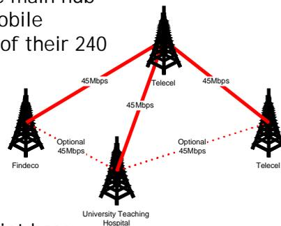
Each tower was provided with a set of point-to-multipoint base stations (BS) from Proxim, also in the 5.8GHz band and with a maximum throughput each of 20Mbps. Each base station covers an area of approximately 60° and each main site has from two to six base station, to cover a sector from 120° to 360°, depending on the physical location of the clinics it serves.
