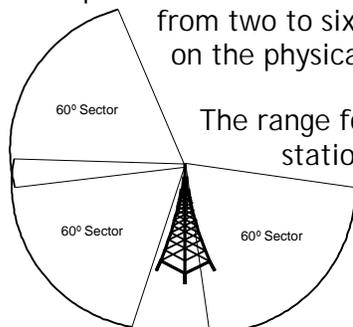
The range for each base station (10 Kms.) was appropriate for most base-station-to-subscriber-unit link, but since this band requires unrestricted line of sight (LOS) and since some places were located near the maximum reach of these units, additional PTP equipment had to be installed to ensure proper coverage of all the clinics. The Quickbridge units from Proxim
