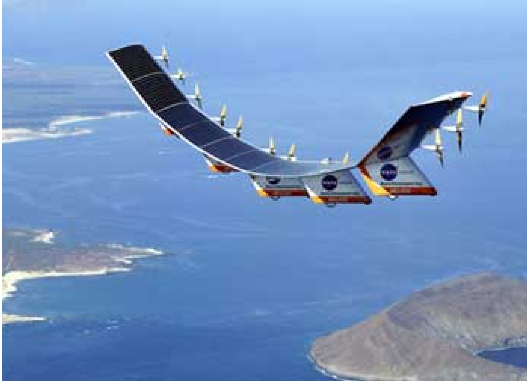
Figure 6. Radio-controlled, solar-powered Helios prototype during its test flight over the Hawaiian Islands on 14 July 2001. (From NASA Dryden Flight Research Centre Photo Collection. Courtesy of NASA.)
