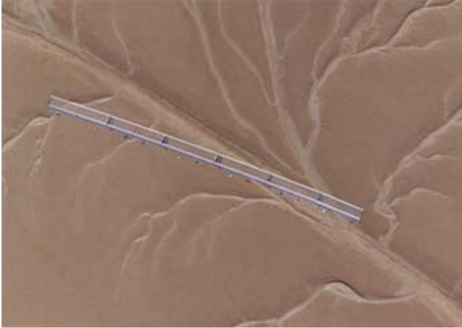
Figure 7. Helios Prototype in flight over a dry streambed viewed from the above. The transparency of the wings with photocells is visible. (From NASA Dryden Flight Research Centre Photo Collection. Courtesy of NASA.)
