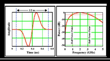
A MONOCYCLE PULSE IN TIME AND FREQUENCY DOMAIN
