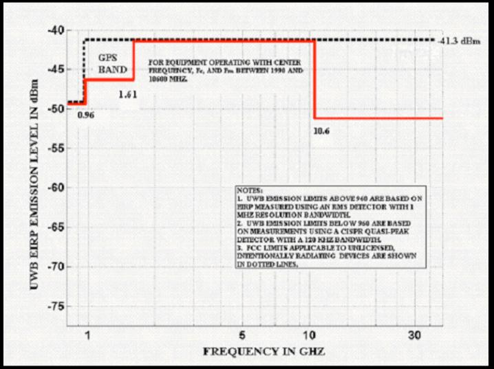
EQUIPMENT OPERATING BETWEEN 1990 AND 10600 MHz WITH CENTER FREQUENCY,  $F_c$ , AND MAXIMUM EMISSION FREQUENCY,  $F_M$
