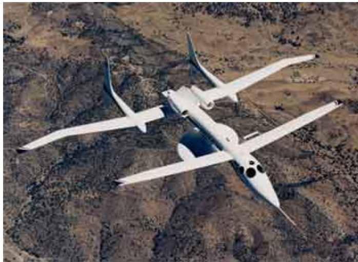
Figure 4. Proteus aircraft, version adapted to serve as stratospheric-altitude communication platform. A disk-shaped antenna is visible below the aircraft's body.
