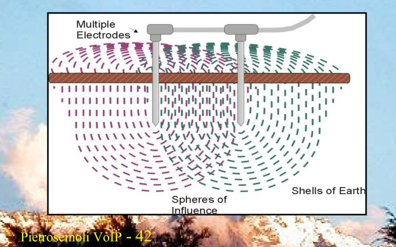
Grounding & Bonding When using multiple rods, they must be spaced apart further than the length of their depth. This will maximize each rod's sphere of influence, thus lowering the total resistance.
