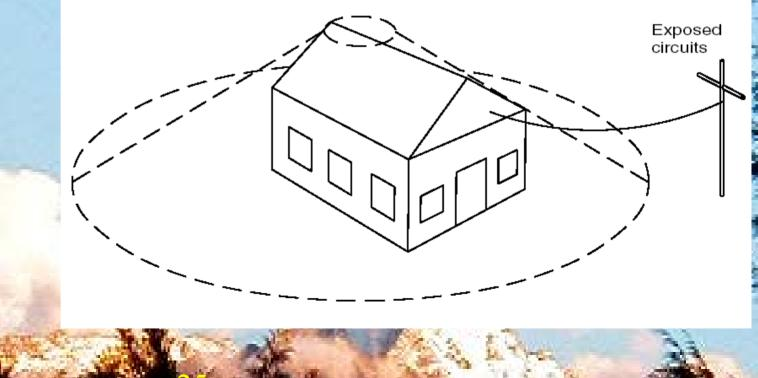
**Protection Systems** Lightning Protection System Multiple rooftop air (lightning) terminals Down conductors Equalizing conductors Air terminals that surround a building for the exclusive purpose of intercepting, diverting, and dissipating direct lightning strikes
