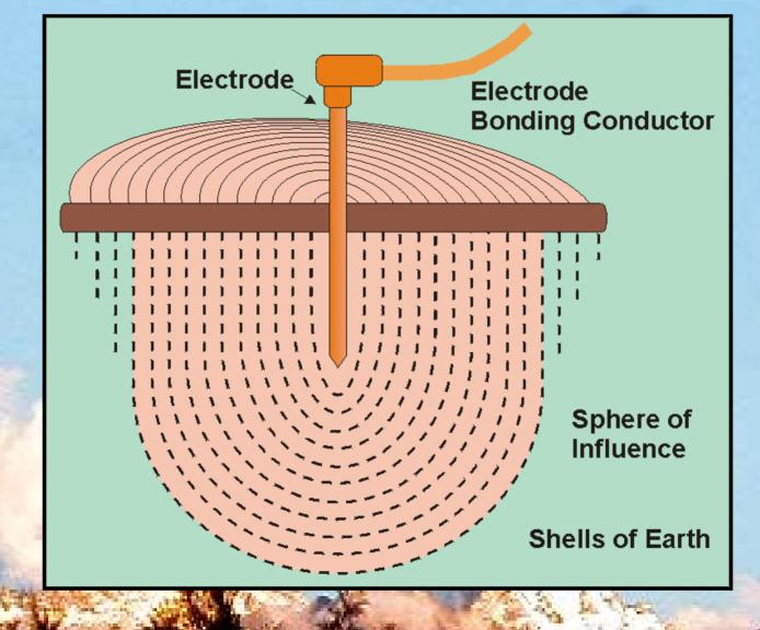
Grounding & Bonding The resistance of the surrounding earth will be the largest of the three components making up the resistance of a ground connection.
