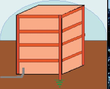
**Building Steel** Usually a very good electrode Large physical size provides low impedance to earth Not always bonded together
