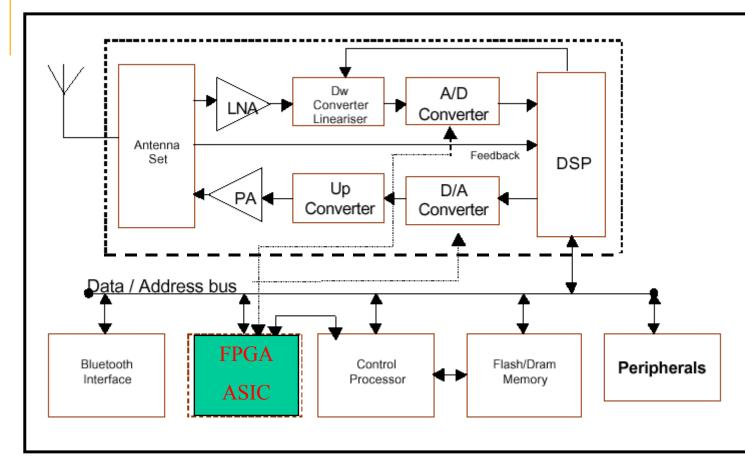
The core of the system is the DSP, responsible of most of the baseband processing; the support of dedicated FPGAs or ASICs for particular heavy computational operations like rake-decoding/Interference mitigation can be necessary depending on DSP computational power. In this last case, a dedicated bus between the DSP and the ASIC could also be needed, or the ASIC should directly communicate with the AD/DA converters and then with the DSP.
