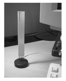
Use the Range Extender Antenna when the integrated antennas of the PC Card are concealed or shielded, for example:
