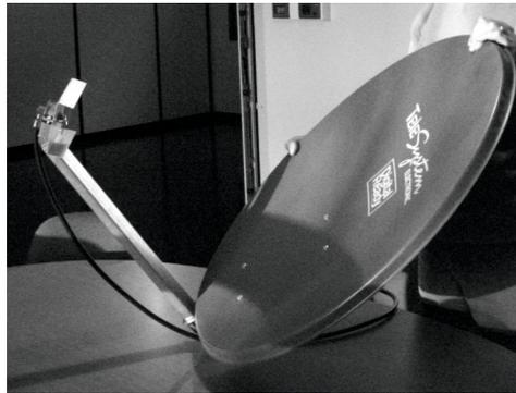
The construction is the same as the stand-alone Biquad antenna, but the shape of the metallic plate is different. The reflector has two side 'lips' which are 3 cm high, used to minimize coupling with the mounting bar of the feeder. These lips cut down radiation from the rear lobes of the biquad.
