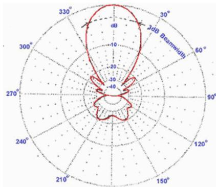
A modified logarithmic scale emphasizes the shape of the major beam while compressing very low-level ( $>30$  dB) sidelobes towards the center of the pattern.
