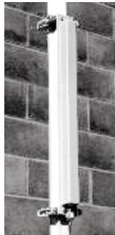
**Panel or Patch antennas:** they are solid flat panels used for indoor coverage, with a gain up to 20 dB.
