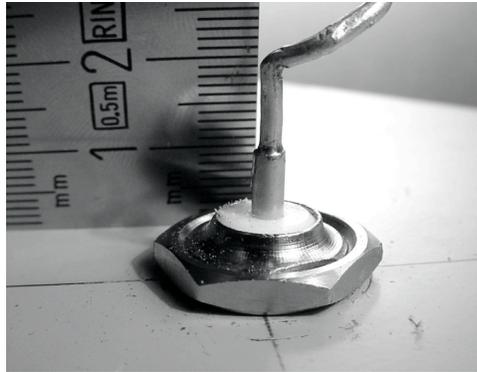
11) We are now going to stretch the coils extending the total vertical length of the wire. Using the use the vice and the pliers, you should pull the cable so that the final length of the coil is of 2.0 cm.
