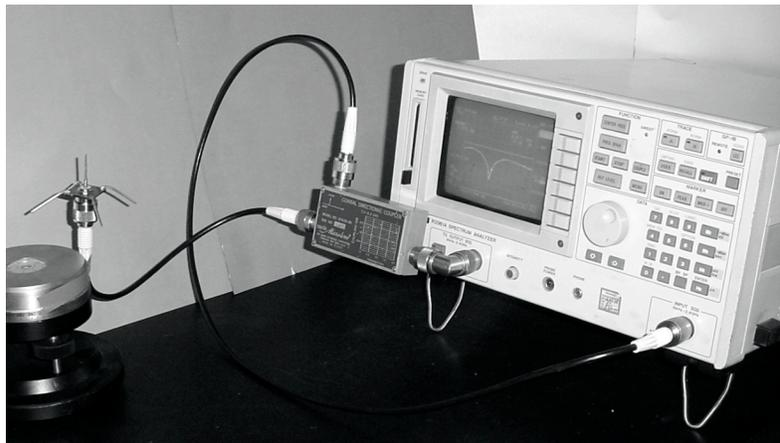
To easily read the value of the reflected power, a calibration of the Spectrum Analyzer is required. In a first step, the reflected power when no antenna is connected to the output port of the Directional Coupler should be measured, and this value should be set as the reference value. In a second step, the power reflected by the antenna under test should be measured. In this way, we measure how much lower the reflected power is, in comparison to the case in which all the power is reflected.
