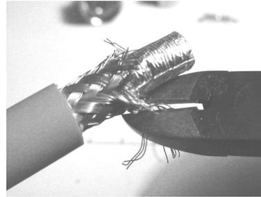
3) Cut the dielectric with the cutter for a length of 'c' mm. Do not nick the center conductor. Tinning of center conductor is not necessary if contact is to be crimped. For solder method, tin center conductor avoiding excessive heat.
