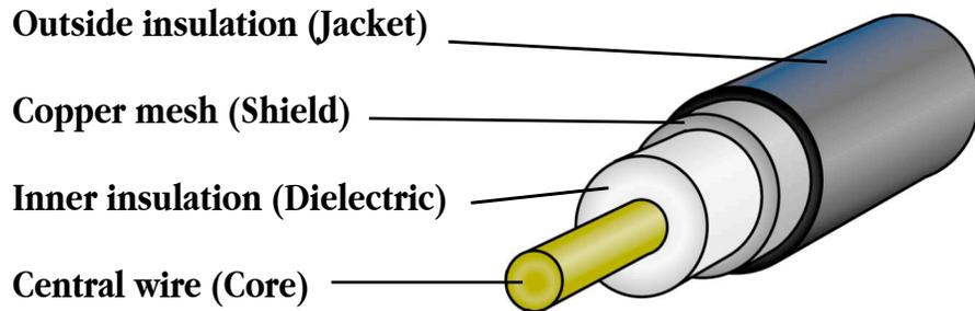
In the following table the diameters of Core, Dielectric, Shield and Jacket of the most popular Coax cables can be found.
