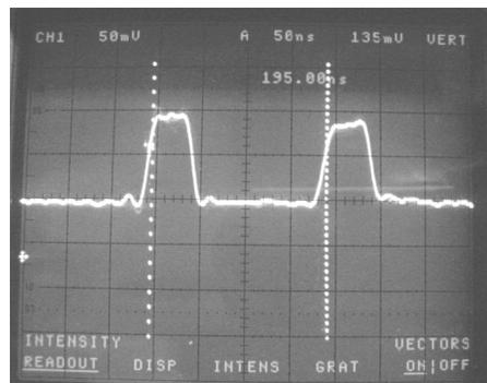
By analyzing the magnitude and shape of the reflected waveform, you can determine the nature of the impedance variation in the transmission system. Also, since distance is related to time and the amplitude of the reflected step is directly related to impedance, the comparison indicates the distance to the fault as well as the nature of the fault. In addition to this, time-domain reflectometer also reveals the characteristic impedance
