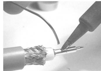
6) Insert the cable into the connector body so the inner portion slides under the braid. Push cable assembly forward until the pin snaps into place. You should hear a 'click' sound.
