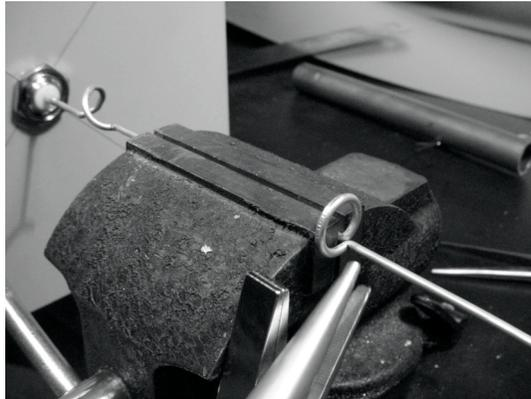
13) At the end the antenna should measure 41.5 cm from the plate to the top.
