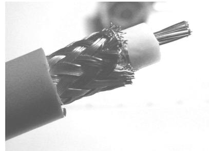
4) Slide outer ring onto cable as shown. Do not comb out braid.
