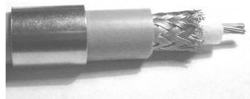
5) Place the central pin on cable's center conductor so it butts against cable dielectric. Center conductor should be visible through inspection hole in the central pin. Solder (or crimp) the pin in place. Do not get any solder on outside surface of the pin. Avoid excessive heat to prevent swelling of dielectric.
