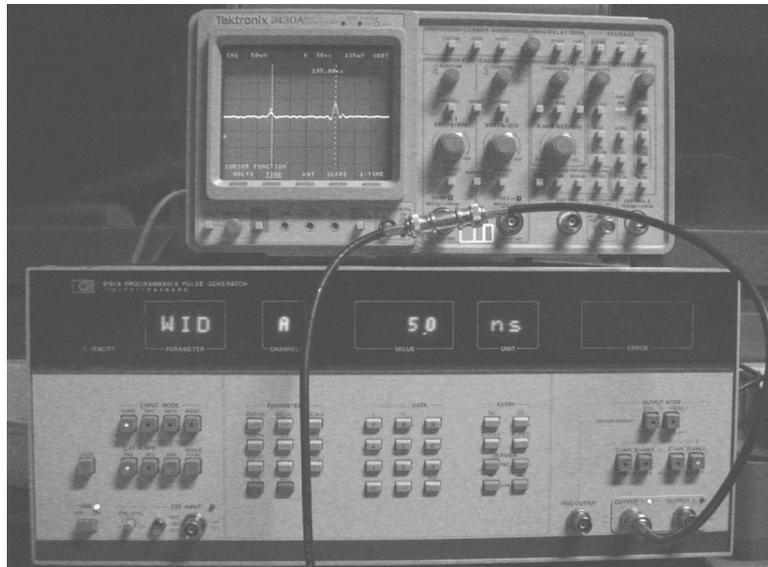
The generator sends a sequence of pulses down a transmission line, and with the oscilloscope it is possible to sample the signal and observe the incident and reflected pulses. When the fast-rise input pulse meets with a discontinuity or impedance mismatch, the resultant reflections are compared in time and amplitude with the original pulse.
