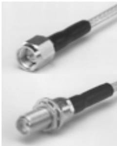
*SMA* is an acronym for SubMiniature version A and was developed in the 60s. 50  $\Omega$  SMA connectors are precision, subminiature units that provide excellent electrical performance up to 18 GHz. These high-performance connectors are compact in size and mechanically have outstanding durability.
