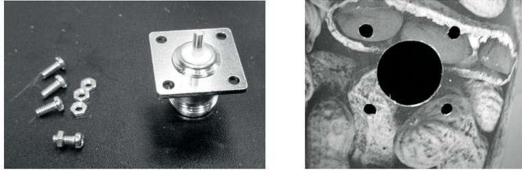
You should also use some additional washers (or thin metallic plates) in order to fit the flange on the curved surface of the can without changing its shape.
