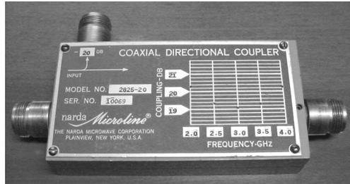
A *unidirectional coupler* has available connections for extracting only one direction of transmission; a *bidirectional coupler* has available terminals for extracting both directions.
