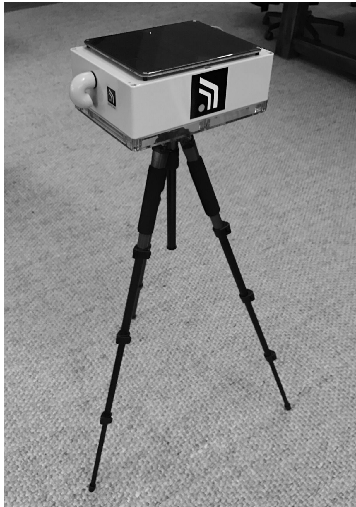
SOLARCAST - stand-alone radiation and air-quality sensor
