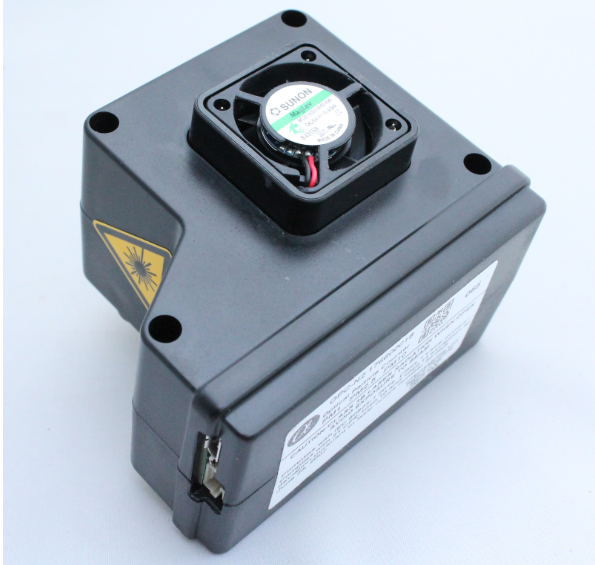
Alphasense Particulate Monitor (OPC-N2)
