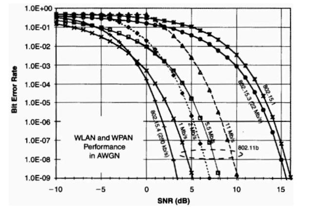
**BER versus** SNR for the four data rates of WiFi (IEEE 802.11b) along with values for **Bluetooth (IEEE** 802.15.1), WiMedia (IEEE 802-15.3) and ZigBee (IEEE 802.15.4), all operating in the 2.4 GHz band
