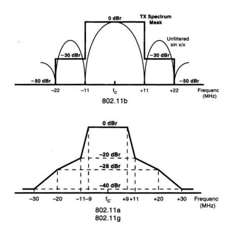
Spectrum masks for WiFi – examples of the projection of multidimensional signal solid onto the Frequency-Power plane
