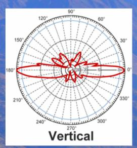
A self supporting tower very often has a tapered design, becoming narrower with height. This will uptilt the beam of a side attached omni up to 5 degrees. A typical 15 dBi omni has an 8 degree vertical beamwidth. The beam can be tilted upwards so much as to send all the signal where it does no good.
