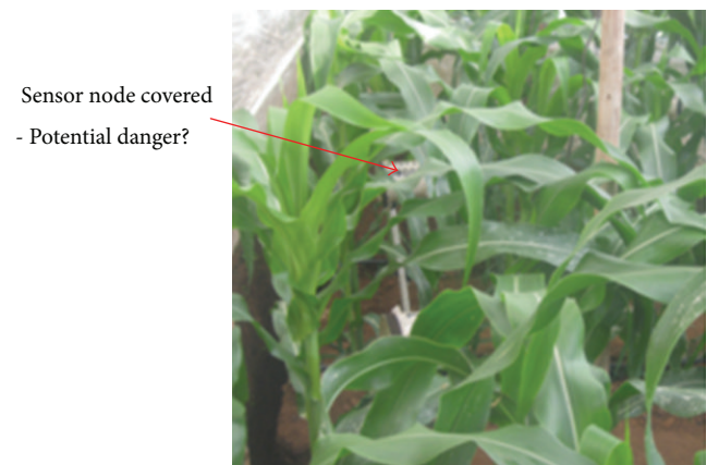
FIGURE 13: Sensor node being covered by maize plants.
