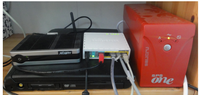
Fig. 3. Indoor hardware of a community network node with router, server and cloud resource
