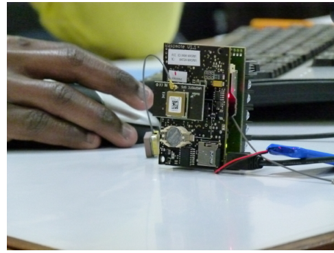
Fig. 2. The Wasmote from Libelium with a GPRS board and Weather Station module.
