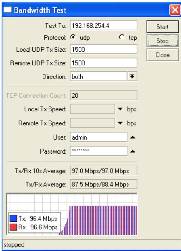
Figure 6: Bandwidth test with the Alcoma link over 15 km of open sea.
