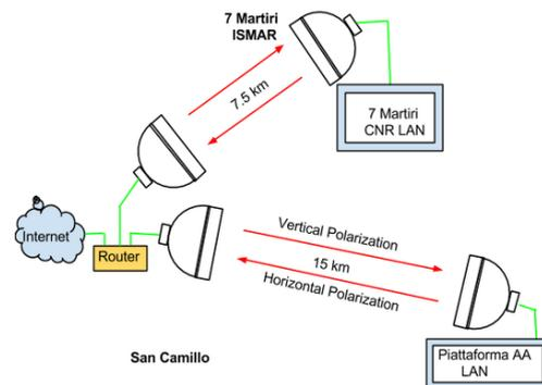
Figure 5: Diagram of the link between the Piattaforma AA and the CNR office at 7 Martiri.
