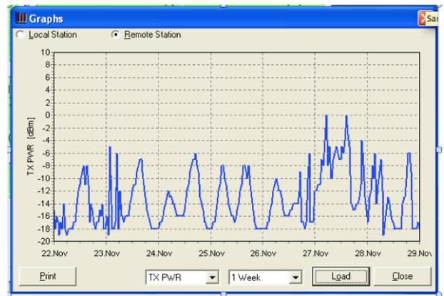
Figure 7: Output power fluctuation to maintain a constant throughput.
