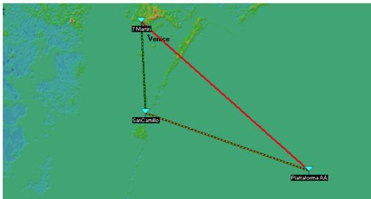
Figure 3: Links from San Camillo to Piattaforma AA and to Riva 7 Martiri. The direct link, shown in red, is obstructed.
