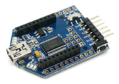
On the USB device, select 5V in order for the WiFi Shield to work!
