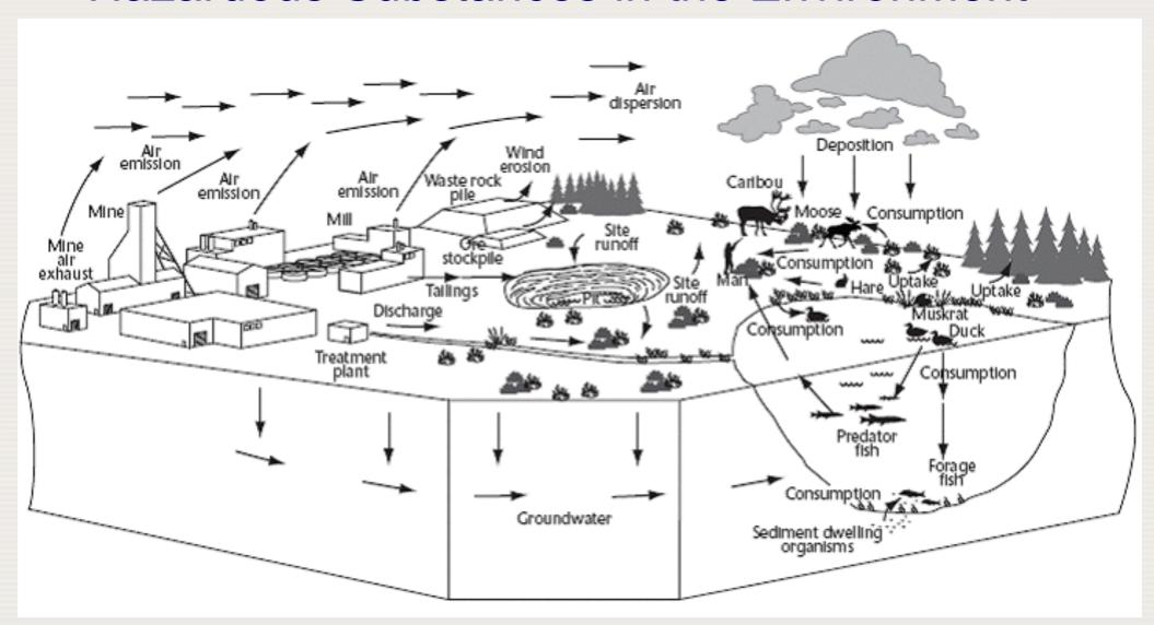
Example of conceptual model for a mining / milling site
