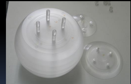
PMMA and PEAD/Pb spheres with dosimeters
